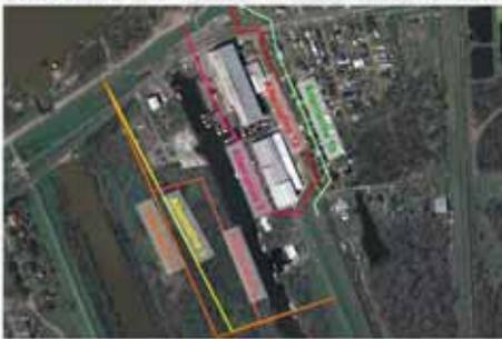
On alternative 1A, we tried staying on the existing alignment. Alternative 1B actually moved towards Degracias Lane, which would have required relocating that entire street. We looked at going west of Elevated Boats, Inc. which in and of itself from a construction stand point is quite problematic. We then started looking going across the Caernarvon Canal, we looked at several alternatives over there, in this line as you can see here.
