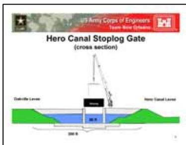
A stoplog gate is constructed in the canal. It's a concrete structure with a 56 foot opening. Traffic would transition through and in the event of a storm this permanently mounted crane would install these stoplogs. They're not wooden stoplogs but metal box trusses. There are two or three stoplogs placed into special slots that would close the canal.
