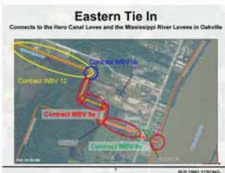
The Easter Tie-in project is composed of three contracts that we internally call WBV, which stands for West Bank & Vicinity, so this is WBV 9a, which is our levees; WBV 9b, which is the main interest tonight that is our Hero Canal Closure Structure; and WBV9c, which is the gates that will be across Highway 23. There is also WBV 12, which connects the Hero Canal Closure Structure along the canal to the West Closure Complex.
