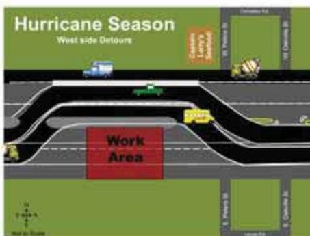
There is a little bit of a switch that will happen when hurricane season starts on June 1<sup>st</sup>, we are required to have two-lanes of traffic in the north-bound direction because Highway 23 is a major evacuation route for this area. So in the area that we are currently working on June 1<sup>st</sup> we will switch to a different traffic pattern as we will have two lanes of traffic going north and a single lane going south.
