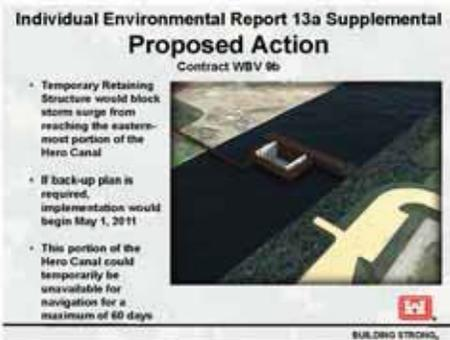
After that, we will be removing this temporary retaining structure. In the unlikely event it doesn't work like it's supposed to, we would have to leave this TRS in place and we would then put the temporary retaining structure that is functioning as temporary flood protection. So what will have is a tie into the levee over here, this TRS here tied into the existing TRS and if that situation happens, the canal is then
