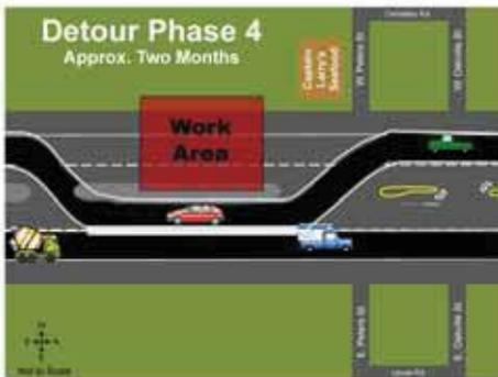
Once we finish this work in this area, we will go to Phase 4, which is basically when the work area shifts to the other side of the highway and we diver traffic with the same idea on the other side of the highway.
