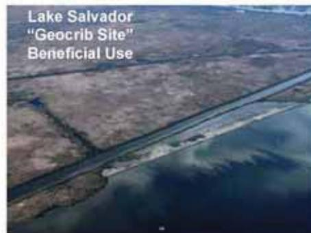
This is just one of the things that we've done. The Algiers Canal is dredged in order to increase the conveyance capacity of the canal to the pump station. The material that was taken out was barged to Lake Salvador, a geocrib site, an area that they have been trying to fill in and rebuild it for a long time. We had this material available so we decided to do some beneficial use of marsh creation in that location in cooperation with the National Park Service.
